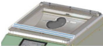
As a final step the SealSafe instrument seals the specimen bag. Fixative injection and sealed are completed in the closed and ventilated cavity.
