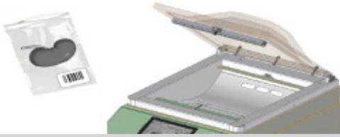
Close the lid of the cavity (you can reseal the bag using it from the operating room through storage).
