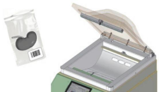
**1 - Place specimen in the vacuum bag and put it inside the instrument cavity**
