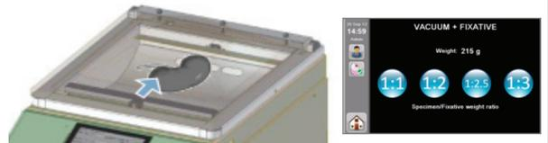
The SealSafe automatically dispenses and injects a measured volume of formalin according to the weight of the specimen.
